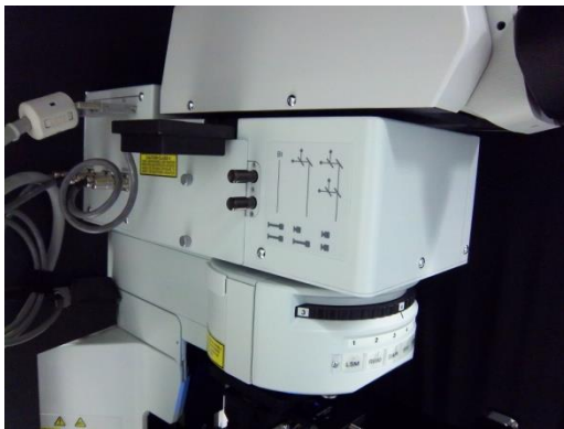
Light to detectors, SDM570 engaged RXD1 (CFP), RXD2 (YFP), and RXD4 (RFP) available.
